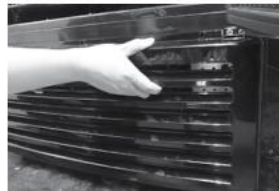
3 The front grill can now be removed by pulling it up.
