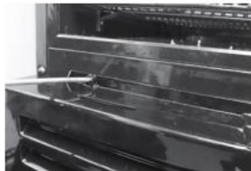
2 Using a small Phillips head screwdriver and remove the screws as shown.
